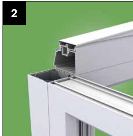
2 Firrings are supplied in one of 2 standard lengths. When cutting the furring, always do this at the back (rear) and ensure that all elements are aligned.
